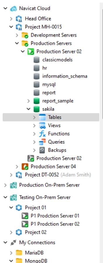
Table elements, such as fields, indexes and foreign keys, are display under each table. Click the arrow to the left of the table name to expand the list. If the elements are hidden, enable the **Show objects under table in navigation pane** option in the [Options](#) window.
